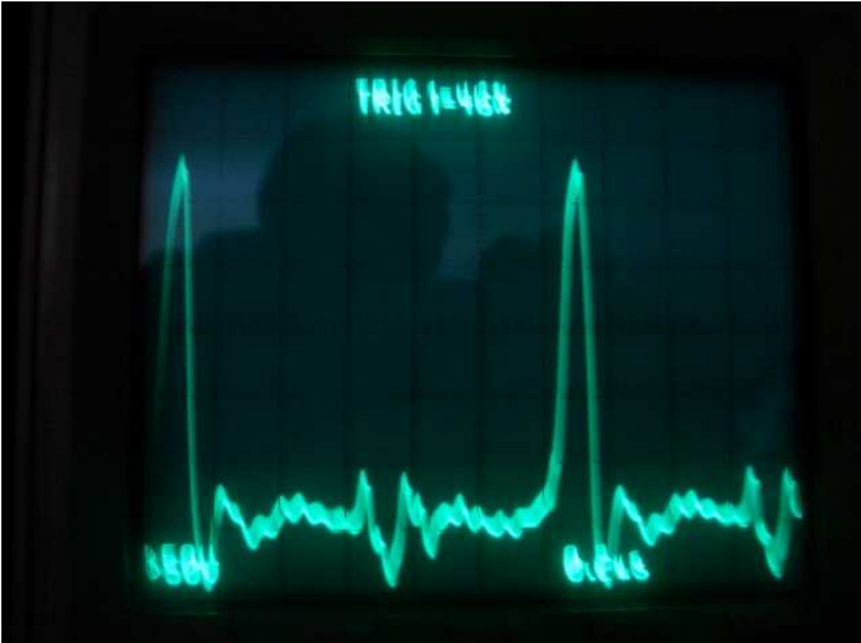
Waveform on Inner Collector Coil under light-bulb load (50V/div)
