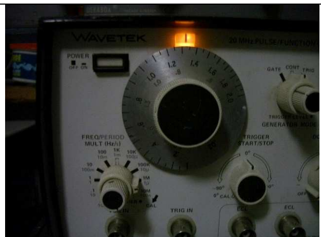
Main Oscillator settings (1.33MHz)
